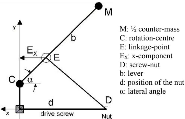
Figure 9: One side of the lever mechanics
