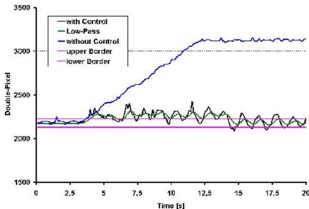
**Figure 13: Transport of a load with and without feedback-control**
