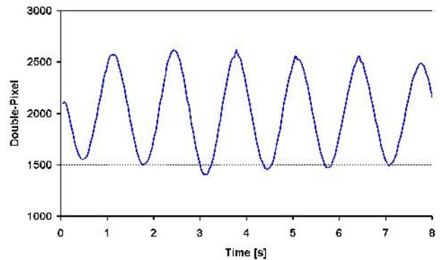
Figure 11: Natural oscillation frequency of the system
