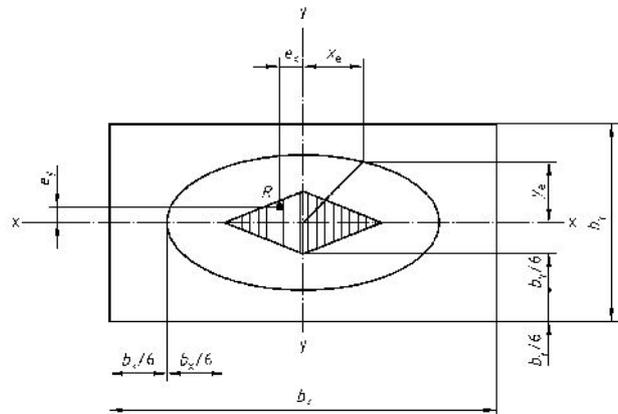
Figure 1: Tolerance region for the centre of gravity /1/
