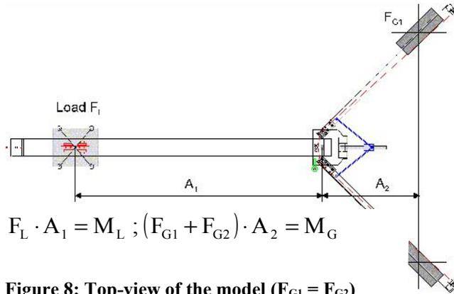
Figure 8: Top-view of the model ( $F_{G1} = F_{G2}$ )
