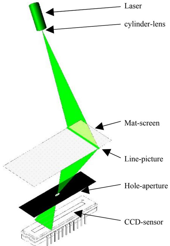
**Figure 6: Schematics of the optical path**
