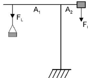
**Figure 3: Principle of torque-free pillar**
