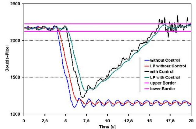
Figure 12: Lifting of a load with and without feedback-control
