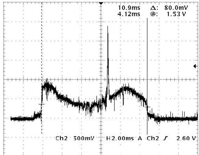
**Figure 7: CCD-sensor-signal (2048 pixels in 10.9 ms)**
